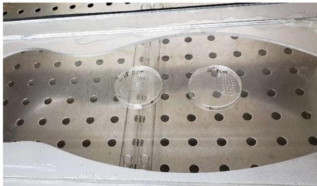
**3 exposure times** to ultraviolet light were tested: 10, 20 and 30 seconds. **Two different samples** located 0 and 8 cm away from the lamp were used for each exposure time.
